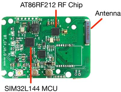
Fig. 1: Custom sensor platform.
