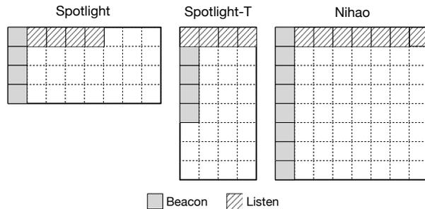
Fig. 15: Comparing Spotlight, Spotlight-T and Balanced Nihao at a duty cycle of 25%.
