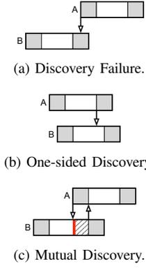
Fig. 6: Three possible discovery cases when two nodes' active slots overlap.
