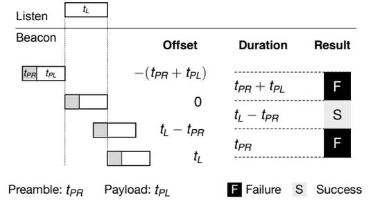
Fig. 10: Discovery failure when preamble falls outside listening period. Note that slot extension still applies.
