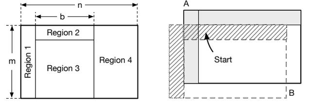
(a) Enumeration of all possible overlap scenarios. (b) Worst-case overlap scenario when  $a = m$  and  $b = n - 1$ . Latency for any valid  $b$  given this offset is  $m \cdot n - 1$  slots.
