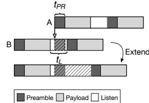
Fig. 5: If B has received A’s preamble, B extends its listening time if necessary in order to receive A’s payload.
