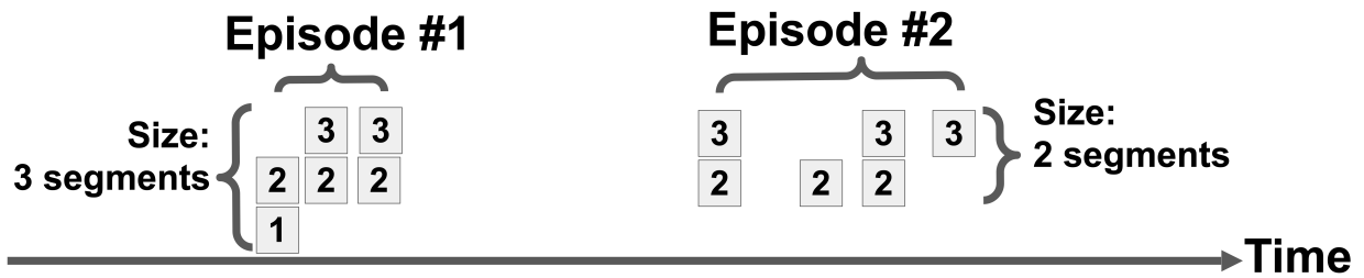
Figure 4.3: Episodes span space (measured in segments) in addition to time. An episode’s size is the smallest number of segments required to be admitted to get all possible hits within an episode. OPT-Range (§ 4.4) is (1,3) and (2,3) respectively.
